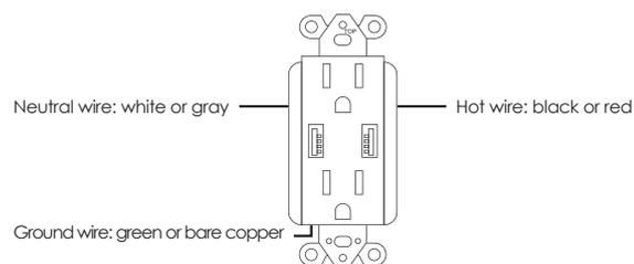
7. Carefully move the new outlet into the wall, with the attached wires loosely bunched behind. Secure the outlet through the slots immediately above and below the outlets with the two included mounting screws (the longer screws). Put the wall plate on the outlet, and secure the wall plate with the two included wall plate screws
