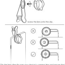
Clip the lens directly over your device's camera lens and ensure the lens is precisely centered on it. You can align them by looking at the device camera lens through the front of the telephoto lens (with the right angle & light). An alternative is to center just the clip first, then carefully screw on the lens. Test the camera to confirm correct fit (a clear view with no black borders or blurred edges). If your device has a case, try removing it for better fit and performance.
